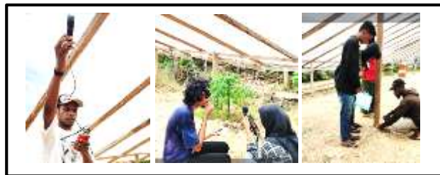
Figure 4. The process of measuring wind speed, temperature, humidity in drying buildings
