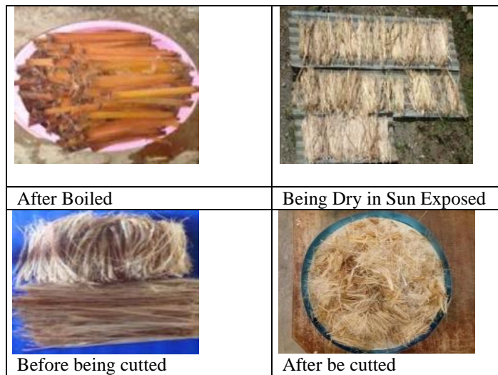
Fig.7. The process of making banana stem fiber.
