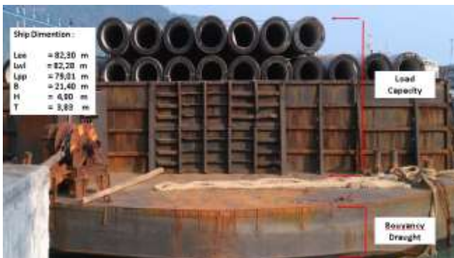
Figure 3. Proses loading unloading at ship
