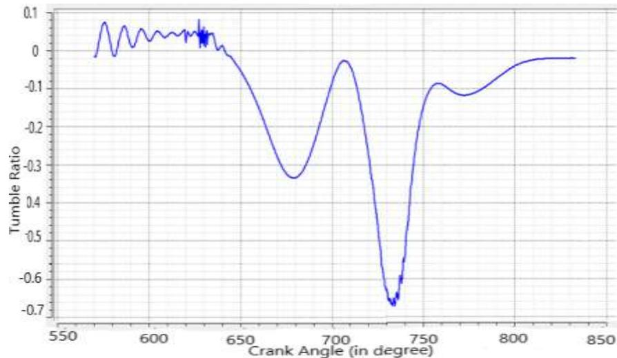
Figure 5. Tumble Ratio Vs Crank Angle
