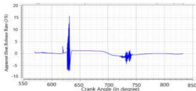
Figure 7. Apparent Heat Release Rate Vs Crank angle
