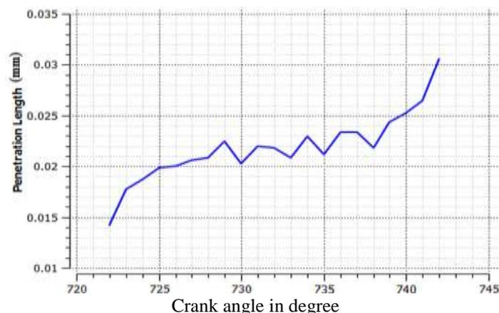
Figure 8. Penetration length of injection Vs Crank angle.
