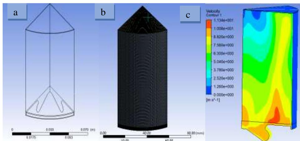
**Figure 1. a) geometry of piston sector, b) mesh of piston sector, c) Velocity Vector Contours**
