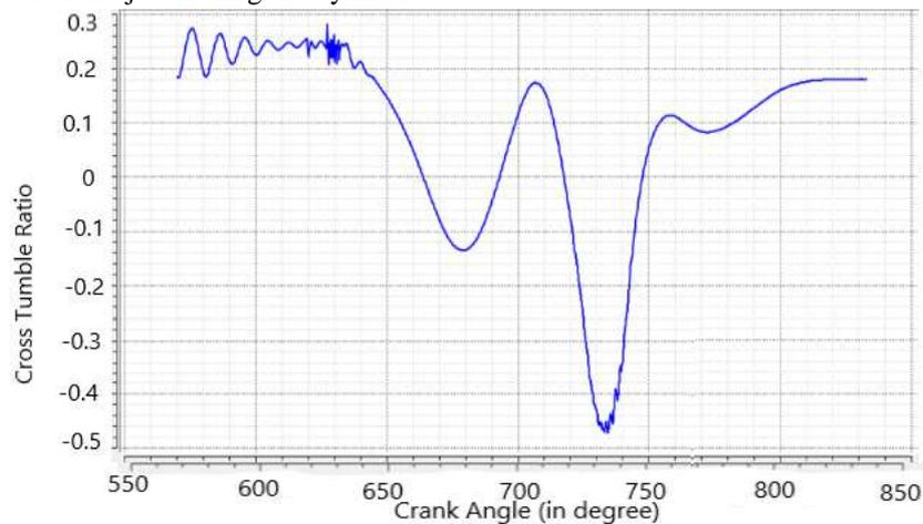
Figure 6. Cross Tumble Ratio Vs Crank Angle
