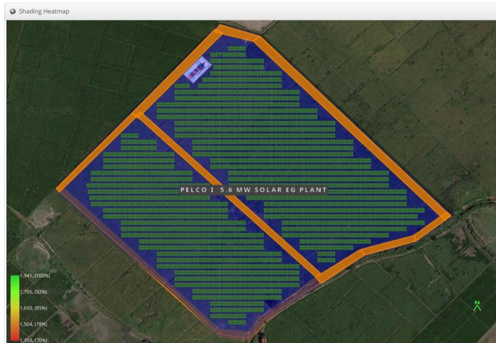
Figure 3.1.1 Proposed Location and Design of the 5 MW Solar EG Plant created using HelioScope Online PV Plant Design Software
