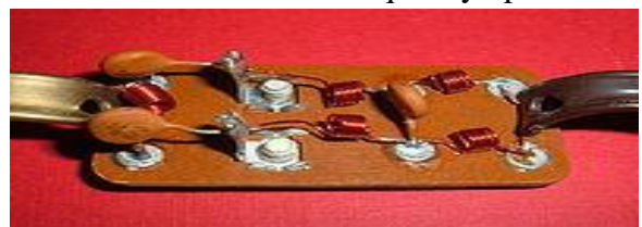
Figure 1: Television signal splitter consisting of a high-pass filter (left) and a low-pass filter (right).
