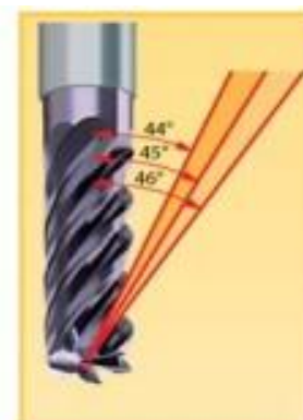
Figure 1. Variable sprain angle of the chip flutes [2].
