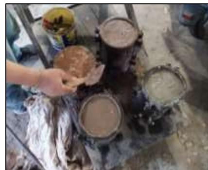
**Figure 2.** Making a Cylindrical Test Object
