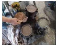
Figure 2. Making a Cylindrical Test Object
