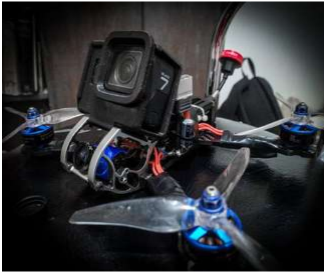
Figure 4. UAV with Portable 5.8ghz FPV system with Smartaudio
