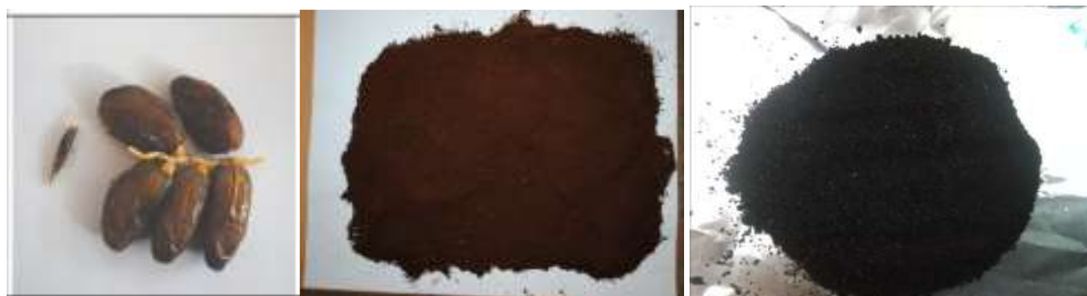
Fig.1. The stages of the preparation and activation of activated carbon from date kernels
