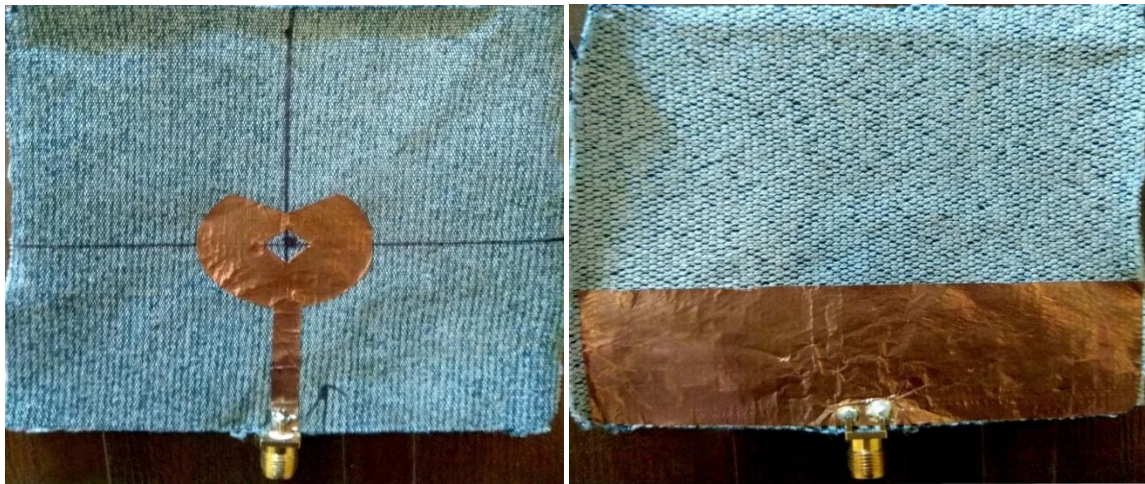
Figure 3: Fabricated circular microstrip textile antenna.
