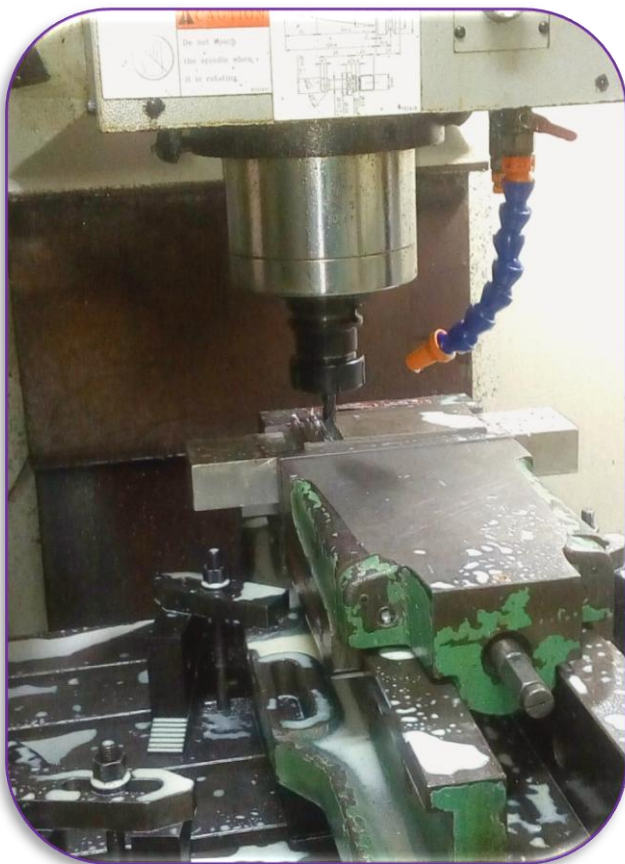
Fig.1a) Experimental setup (CNC Vertical Machining Center, KENT INDIA Co, Ltd, Taiwan)
