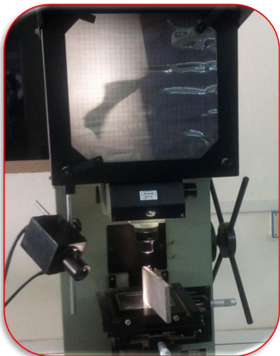
Fig. 2 Profile Projector for measuring Burr size
