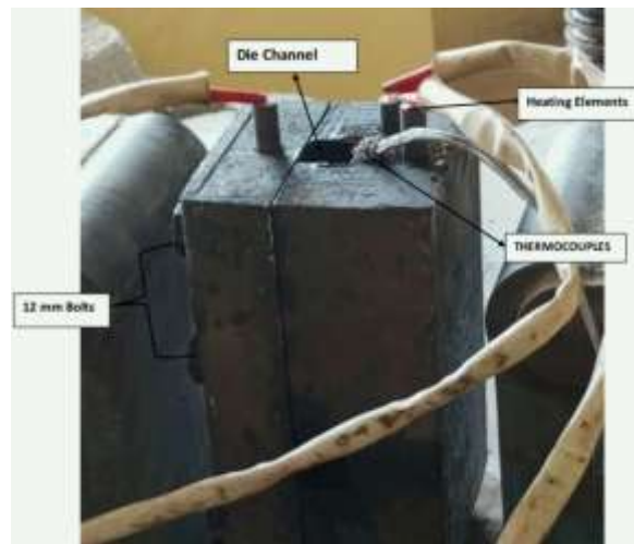
Figure 2: Assembly of ECAP Extrusion Rig
