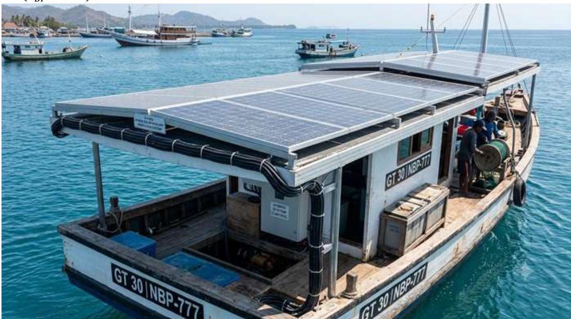
Figure 2 Fishing Vessel 30GT with Solar Panel System
