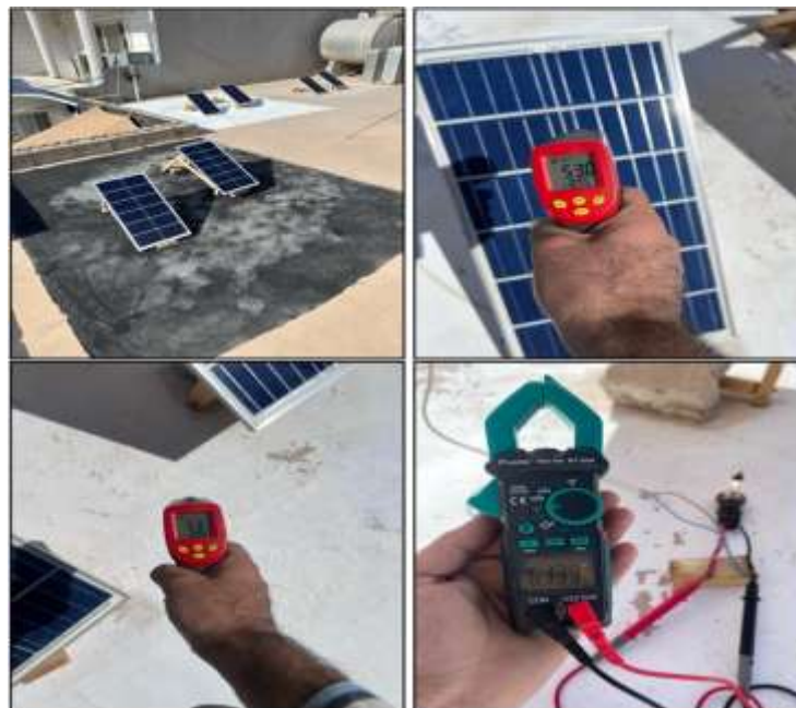
Figure1: Field experimental setup in Kirkuk, Iraq: (a) Rooftop layout displaying monofacial PV panels mounted at a 33° tilt angle facing South over black absorptive and white reflective surface coatings, (b) Surface temperature measurement of the PV module using an infrared thermometer, (c) Thermal logging of the underlying rooftop coating surface ( T_{\text{roof}} ), and (d) Load measurement and electrical parameter using digital multimeter/clamp meter .
