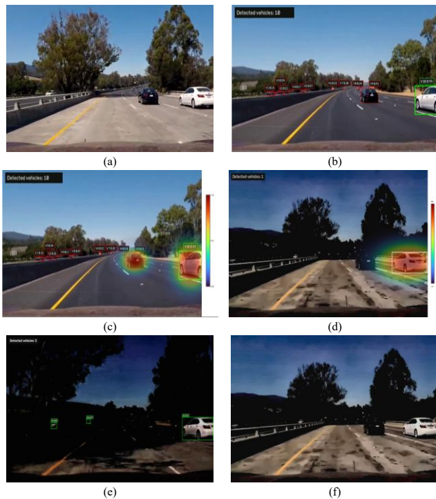
Fig. 1. Vehicle detection in daylight and nighttime simulation. (a) Original daylight image. (b) Detection results of YOLO11s in daylight condition. (c) Confidence weighted heatmap of daylight detection. (d) Simulated image of nighttime. (e) Detection results of YOLO11s under simulated nighttime conditions. (f) Confidence weighted heatmap for nighttime detection.
