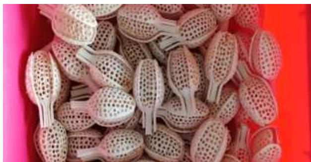
Figure 1 biofilter media made from used plastic spoons
