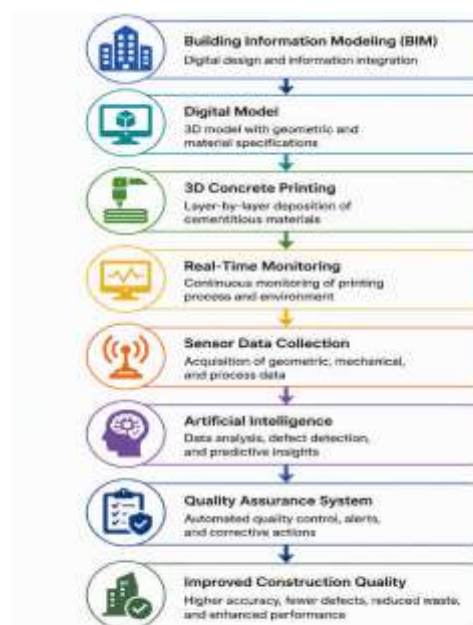
Figure 1. Conceptual framework for quality control in 3D concrete printing.
