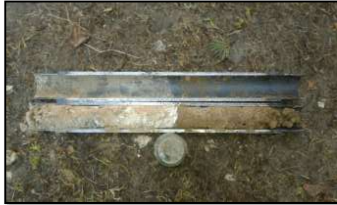
Figure 2. Shelby tube used to collect disturbed soil sample from borehole.
