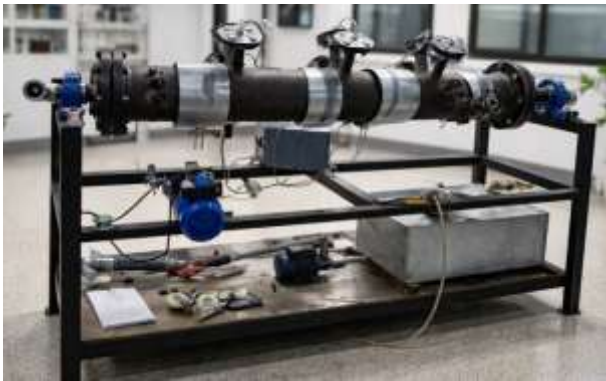
Fig 3: Annular heater connected to the shell.
