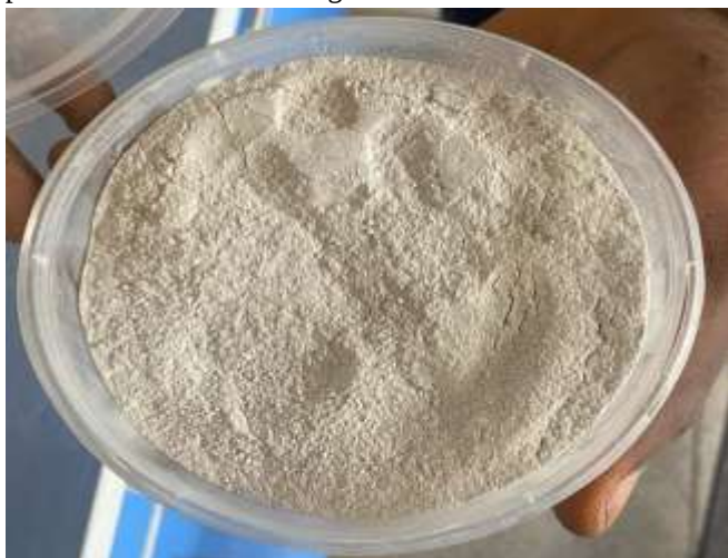
Figure 1: Rice Husk Ash after combustion for 2 hours at 650°C and Sieving
