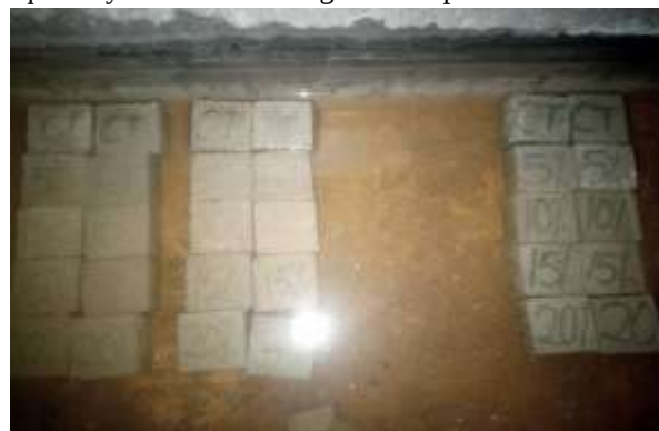
Figure 3: Curing Of RHA-Cement Mold Samples
