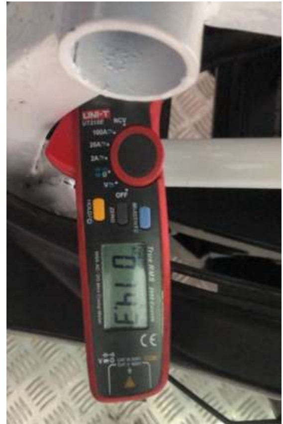
Figure 2. Data collection techniques using ampere meters
