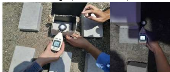
Figure II-15. Light transmission testing of pavement blocks using artificial and natural light sources in a controlled dark box.
