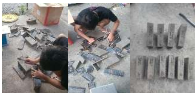
Figure II-10. Dismantling of the formworks
