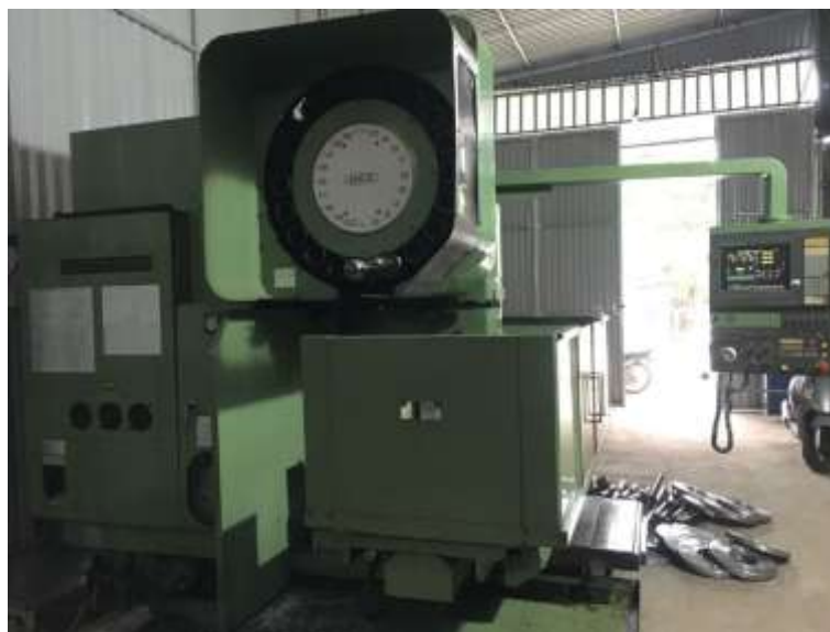
Figure 1. MCV-410 milling machine used for experiments
