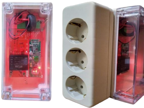
Figure 3 Overvoltage monitoring device and enclosure
