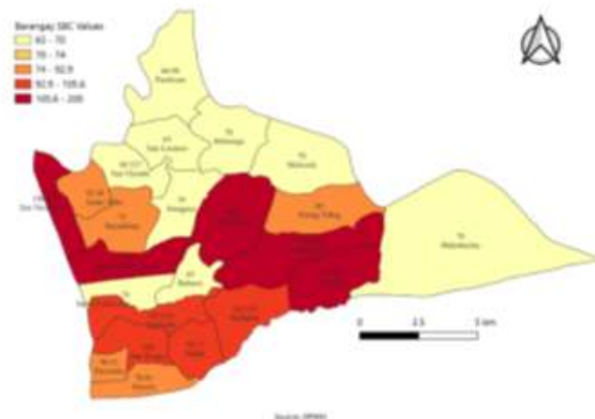
Figure 3. Spatial Distribution Map of Allowable Soil Bearing Capacity (1.5m Embedment Depth)
