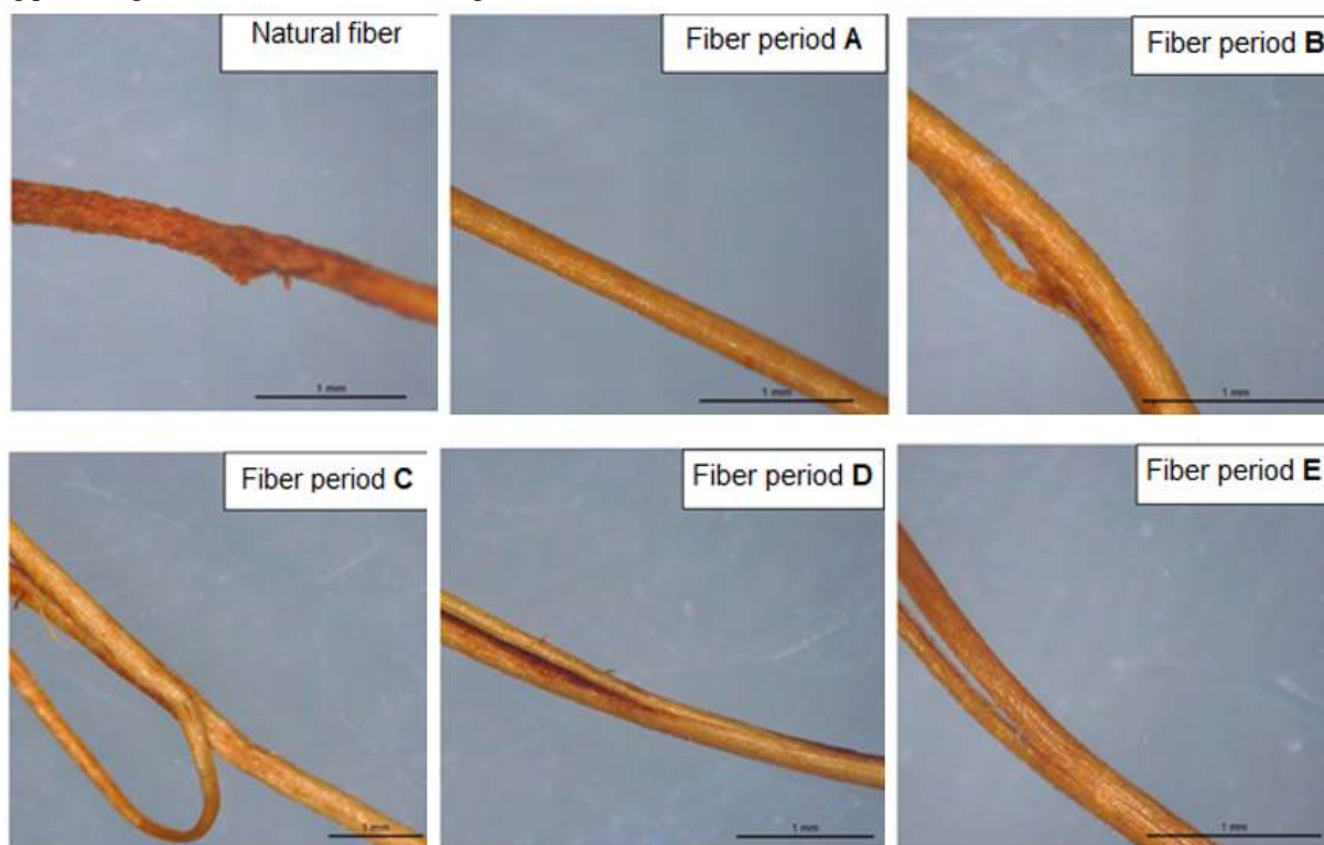
Figure 10-Optical micrograph of natural coconut fiber and after treated with ultrasound agitation at different periods (A, B, C, D and E).
