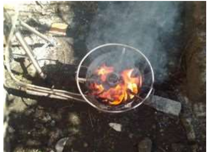
Figure 3. The crucible as positioned in the furnace
