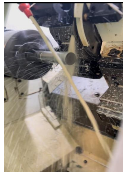
Figure 2 Wet cooling condition
