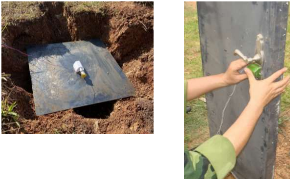
Fig. 12. Installation of the explosive charge on the door-lock system
