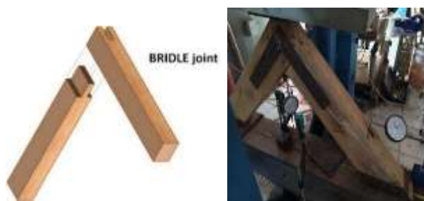
Figure 5. Bridle or Knee Joint of Gmalina arborea
