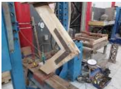
Figure. 8 Test of Wooden Joint with Closed Direction Loading
