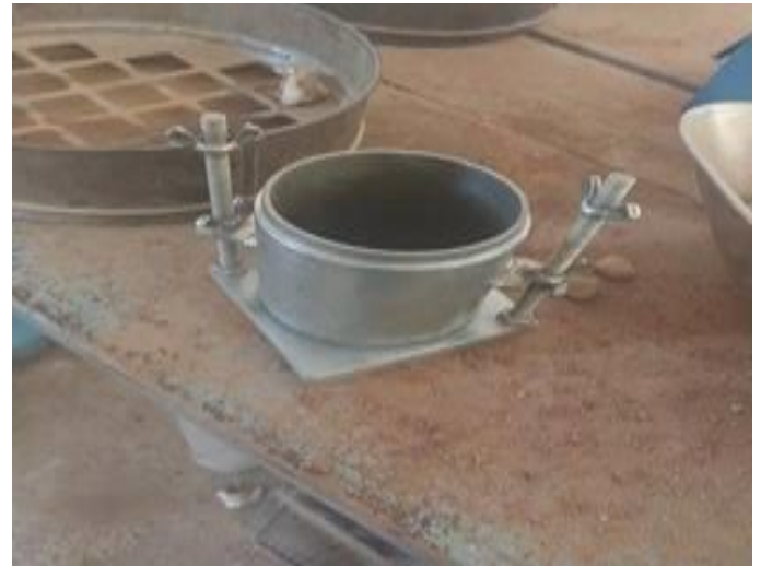
Figure 5. Standard container with known volume used for bulk density determination.
