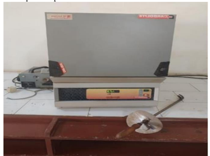
Figure 6. Electric furnace used for alkali fusion treatment.
