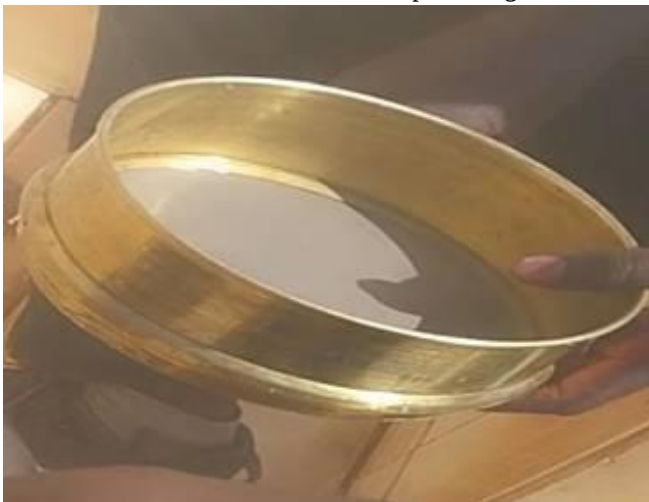
Figure 4. Silt test apparatus used for determining fine particle impurities.
