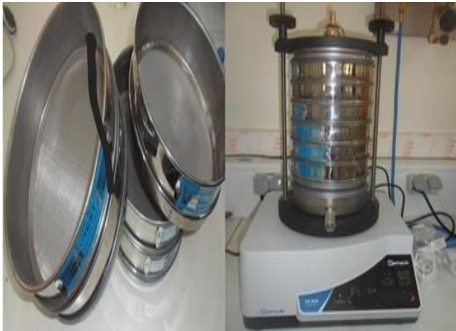
Figure 3. Mechanical sieve shaker and standard sieves used for particle size classification.
