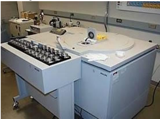
Figure 8. X-ray fluorescence (XRF) spectrometer used for elemental analysis.
