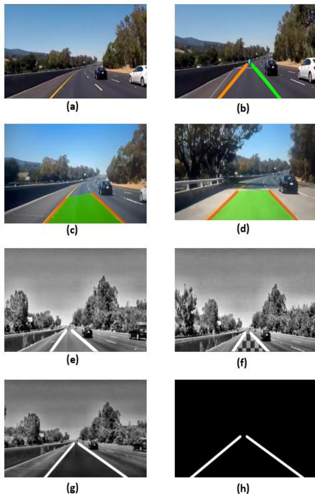
Fig.2. Qualitative results of the proposed lane-detection pipeline in daytime and nighttime conditions (a–h). Daytime examples (a–d) show the raw input, extracted boundaries, and corridor overlay under typical daylight variations, while
