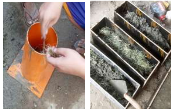
Figure 2. Incorporation of Fiber to Concrete
