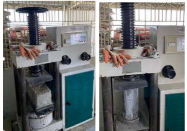
Figure 3. Laboratory testing of concrete specimen under axial compression and flexural strength.
