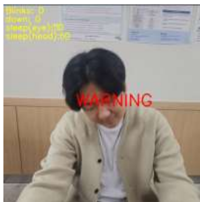
Figure 1. If the driver bows their head for a certain period, an alarm sounds
