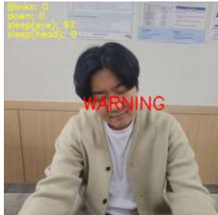
Figure 2. If the driver closes their eyes for a certain period, an alarm sounds.
