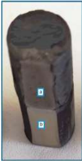
Figure 1. Samples with a diameter of 10 mm and a size of 100 mm; a) Duplex stainless steel, b) AISI 4140 steel
