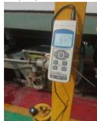
Figure 1. Measurement of solar radiation with the SPM-1116SD solar power meter
