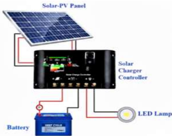
Figure 2. The schematic diagram of the railway signal lamp using solar panels
