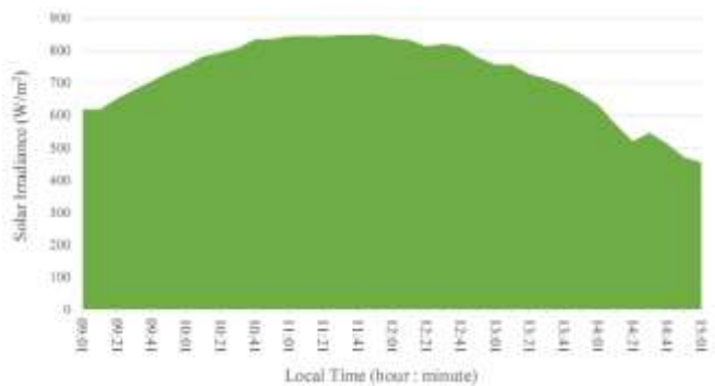
Figure 5. Temporal distribution of solar irradiance measurements at the project site
