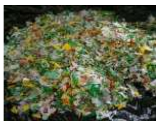
Figure 5 Plastic Waste Shredding Results
