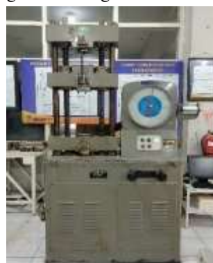
Figure 8 Compression Testing Machine Figure 9 Roster Sample Testing
