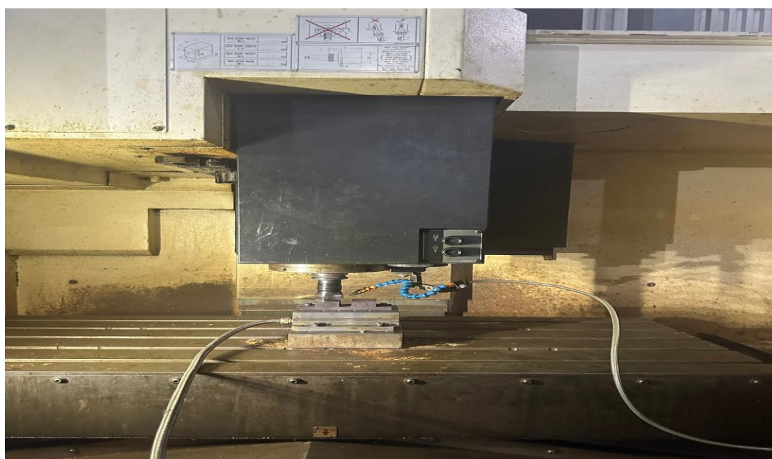
Figure 1. Mazak Vertical Center SMART 530C used for hard milling experiments
