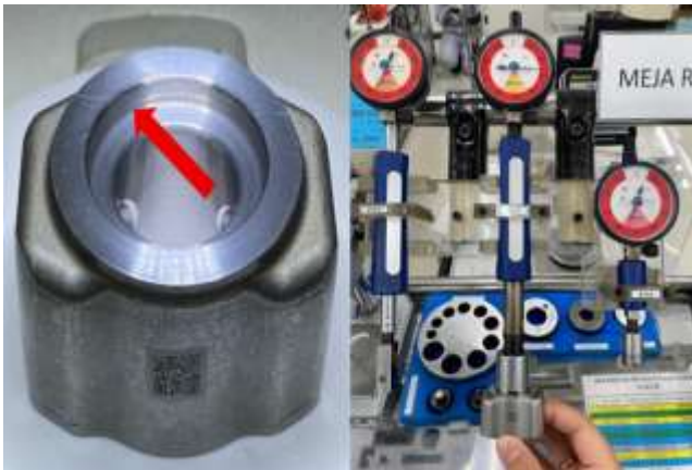
Figure 8. Sunpoudashi defect Source: Data processing, 2025
