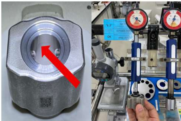
Figure 9. ID 14.8 topatsu defect Source: Data processing, 2025
