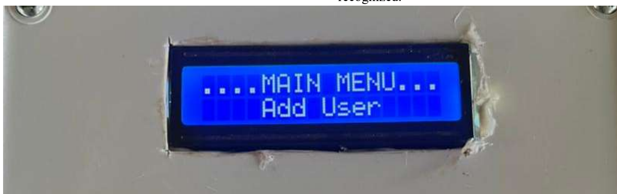
Figure 3.4(a): Adding User through the Smart Cards UID
