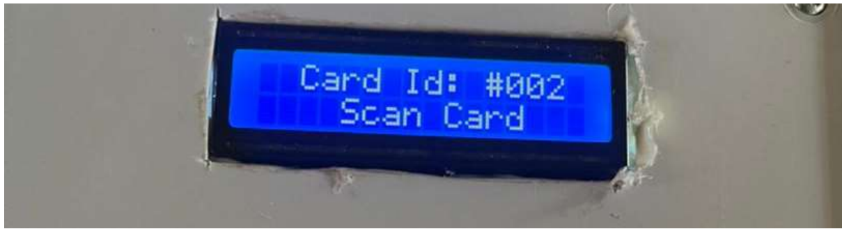
Figure 3.4(b): the system scans the Smart Cards UID to know if the user is registered
