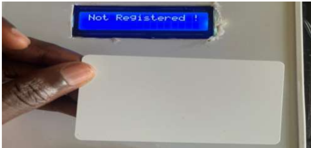
Figure 4.2(b): Display for an Unregistered Card
