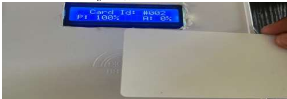
Figure 4.3: Display when the Card is scanned or attendance
