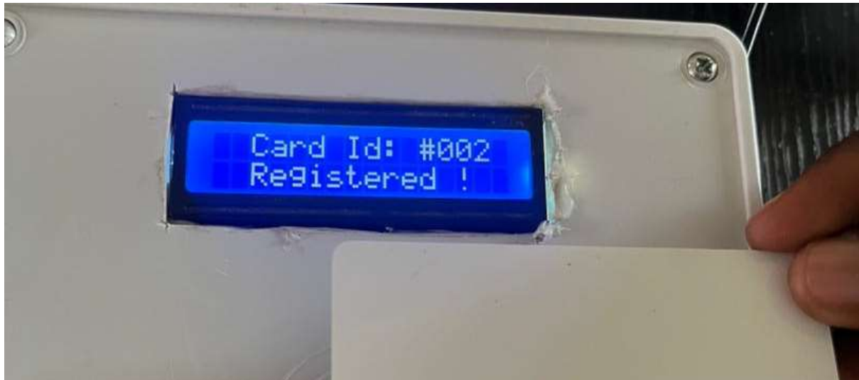
Figure 3.4(c): the system displays Registered, to show that the card is assigned to a student
