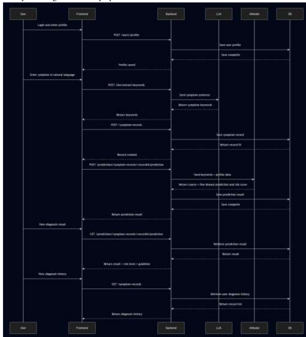
Figure 4 Sequence diagram showing the end-to-end flow of user requests across the system modules
