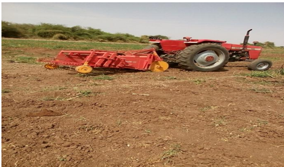
Plate (1) Potato harvesting machine linked to the tractor
