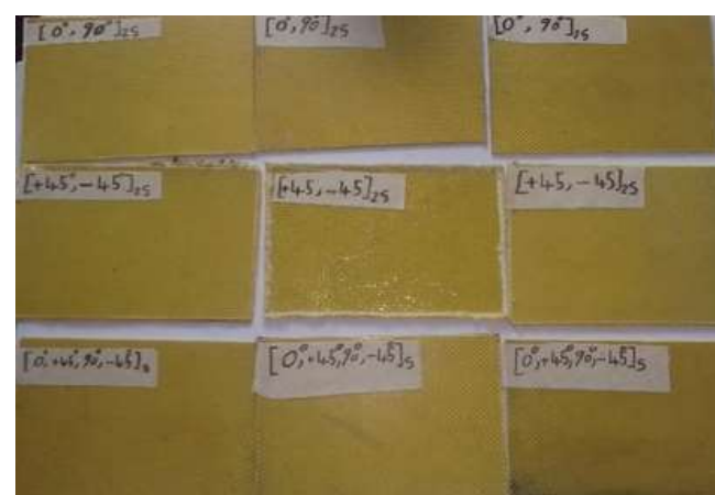
Figure-3 Specimens for drop weight test
