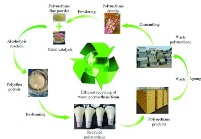
Figure 1: Schematic of closed-loop recycling of flexible polyurethane foam (Gu, et al., 2023).
