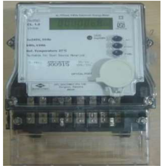
Figure 1: Three-phase electronic digital meter
