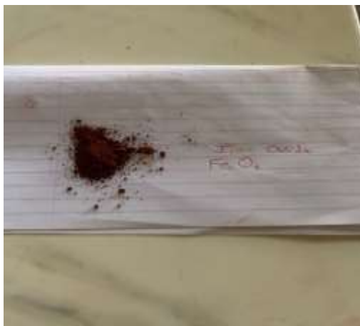
Fig. 2.3 Iron oxide ( \text{Fe}_2\text{O}_3 ) catalyst
