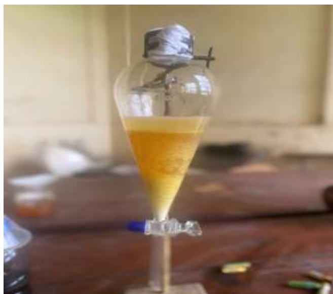
Fig 2.5 Segregation of the biodiesel from the glycerin after transesterification.
