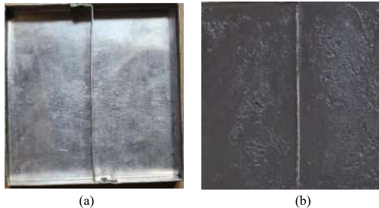
Figure 1. Constructed mould (a), and mould containing developed brake pads (b).
