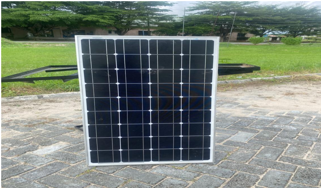
Figure 3. 100Watt PV module
